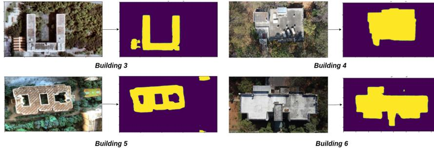
Fig. 8: Roof Segmentation results for 4 buildings.
